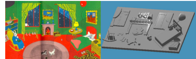
Figure 5. 3D file view for printing tactile pictures
